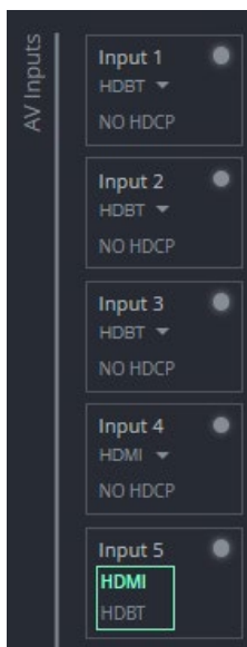
Figure 62: AV Routing Selectable Inputs following HDBT Pre-Configuration
